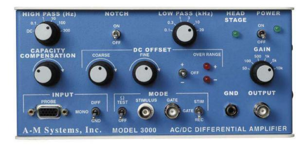
The Model 3000 High-Gain AC/DC Differential Amplifier is a single channel instrument designed for low-noise recordings from excitable tissue. Specific applications include EEG, EKG, extracellular recordings, etc. For users wanting to make extracellular single cell recordings, optional headstages increase the flexibility of this amplifier!
