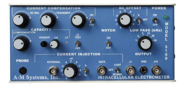
The Model 3100 Intracellular Electrometer is a simple to use, low cost intracellular amplifier. It comes equipped with a small and light weight probe measuring 1.1cm in diameter by 5.6cm long and weighing only 10 grams. This instrument is ideal for research and teaching labs!
