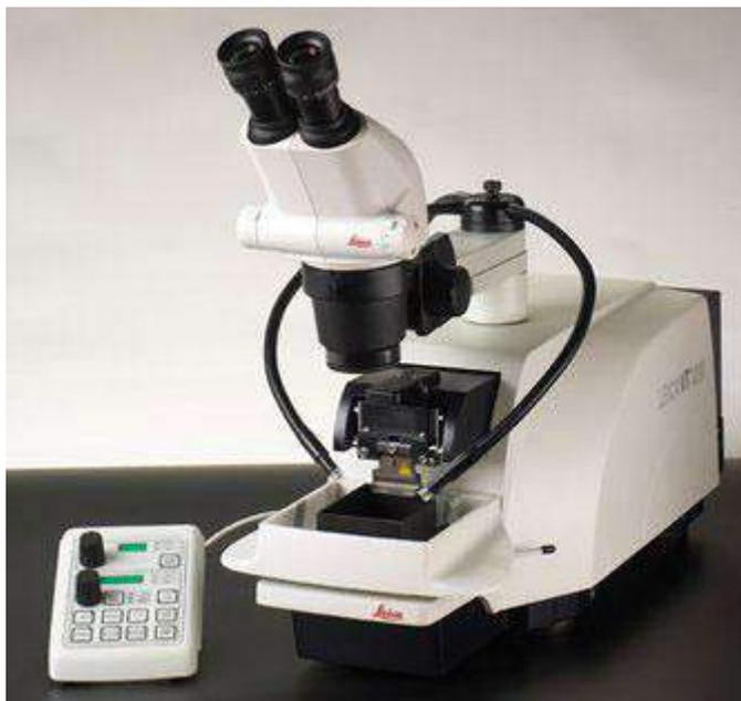
The Leica VT1200 semiautomatic vibrating blade microtome is designed for sectioning fixed or unfixed specimens in Neuropathology (fresh brain slicing), Neurophysiology (patch-clamping).
