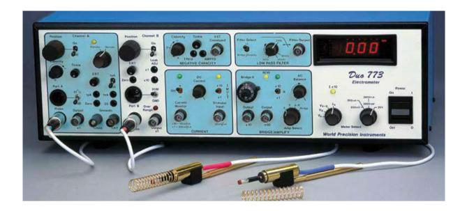
For intracellular dual or differential studies, the Duo773 has separate negative capacity controls and built-in active filtering that allows the precise balancing of time constants for artifact-free differential measurement. Comes complete with two probe headstages, 1015 Ohms & 1011 Ohms probes to monitor signals from ion-specific micro-electrodes as well as KCI-filled electrodes.
