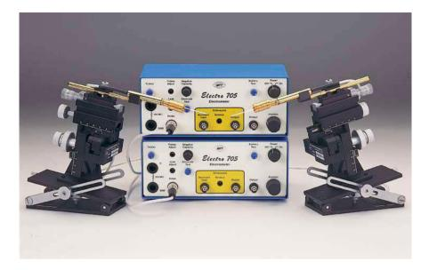
**Remote Headstage** - Easily mounted in any manipulator, this small probe, containing the first stage of amplification, includes a microelectrode holder, which plugs directly into the probe input.
