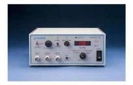
The CL-100 Temperature Controller is an automatic single channel controller capable of accurately maintaining a Peltier device between 0° and +50°C, or a resistive heating element between ambient and +65°C.
